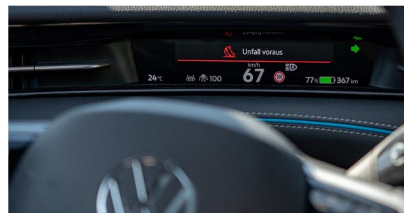
C-ITS Accident Warning in Volkswagen ID.7
